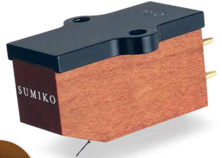
ABOVE: Partially exposed magnet, yoke and coils are mounted onto a rigid alloy top plate (with threaded lugs), while the 90° angles of the plumwood sleeve assist accurate alignment
